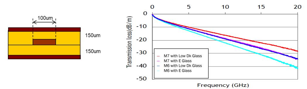
Low Dk glass offer better electrical performance for high speed PCBs due to lower Dk/Df.
