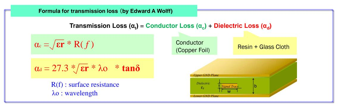
**Reduction of αd :** Lower Dk / Df Dielectric materials **Reduction of αc** : Lower profile or Profile-free conductor
