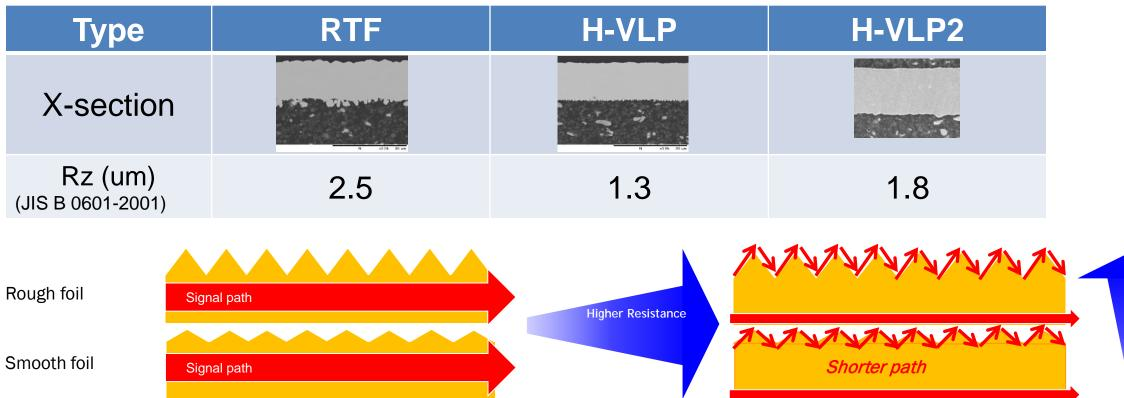
Copper profile is one of the main contributors for transmission loss for high frequency signals.
